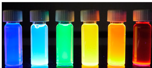
Figure 8. Photograph of 3–4 nm Si-NCs functionalized with various surface groups dispersed in toluene, under UV illumination. From left to right the Si-NC functionalization: blue, dodecylamine; blue-green, acetal; green, diphenylamine; yellow, TOPO; orange, dodecyl (air); red, dodecyl (inert).
